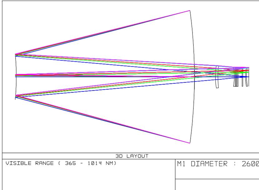
Figure 2-1 VST complete optical layout of telescope with one fixed lens, the ADC and a curve dewar window
