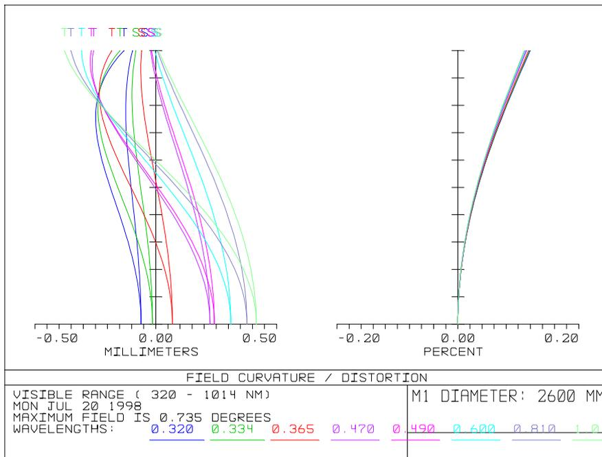
Figure 4-2 Field curvature and distortion curves for the configuration with two lenses
