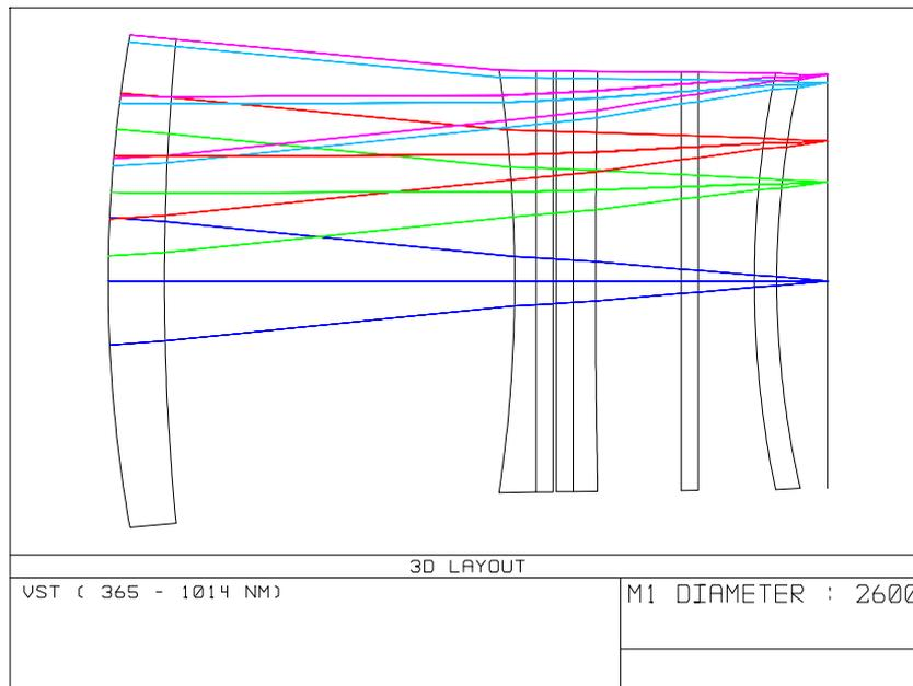
Figure 2-2 VST zoom of the optical layout of the corrector with one fixed lens, the ADC and a curve dewar window
