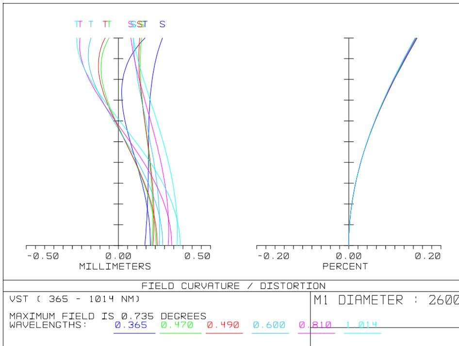
Figure 4-1 Field curvature and distortion curves for the configuration with one lens and ADC
