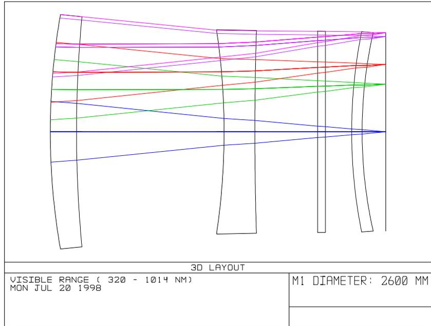
Figure 2-4 VST zoom of the optical layout of the two lenses (U ÷ I bands)
