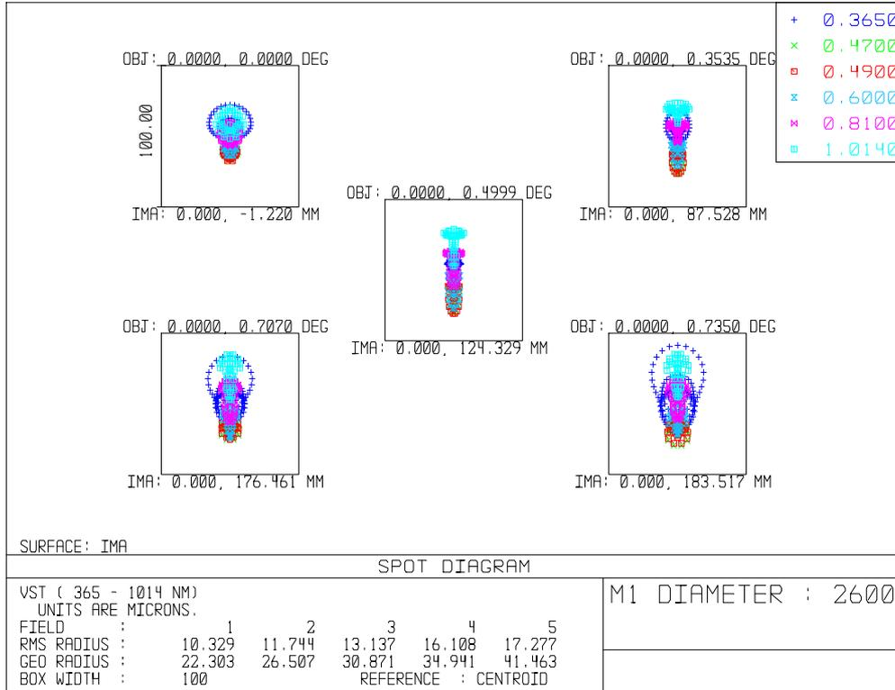
Figure 5-2 Spot diagrams for one fixed lens and ADC at  $z=63^\circ$
