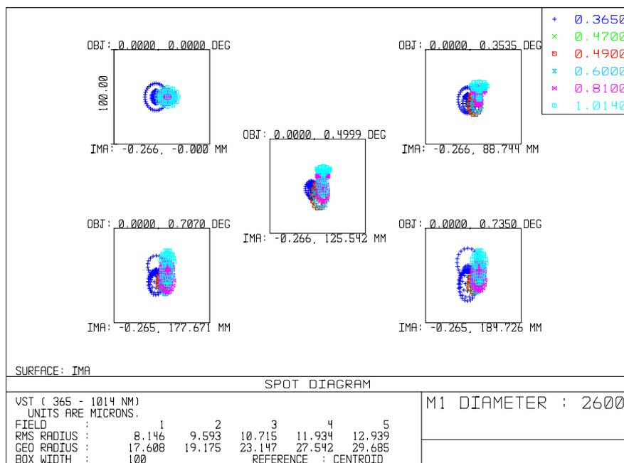
Figure 5-1 Spot diagram for one fixed lens and ADC at zenith from B to I
