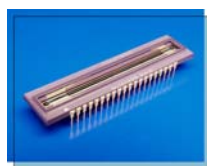
Fairchild linear CCD 191 is a 6,000 element linear CCD with 10 \mu\text{m} pixels. This device offers the ultimate in dynamic range, QE and resolution.
